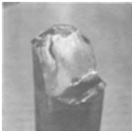
Fig. 18. SR 1855 54 H RC q_{\text{brott}} = 17000 \text{ kp/cm}^2
