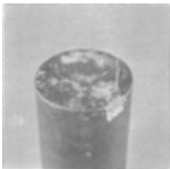
Fig. 19. ROP 57 60 H RC q_{\text{brott}} = 18000 \text{ kp/cm}^2
